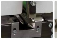
Two finger paper pick-up system allows mixed paper stocks to be handled more easily.
