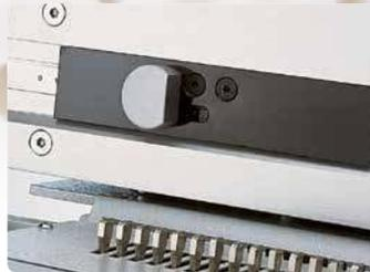
Paper stop with automatic sensor. Activated when the paper is placed in the die and moved over the sensor allowing for fast and accurate punching.
