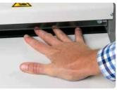
Automatic safety switch will always cut off the machine preventing any injury to a worker. The machine can be easily reset by turning the power switch off and on.
