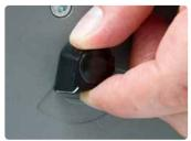
Depth gauge feature allows the operator to adjust the punched hole margin from 2 mm to 4,5 mm. This adds strength to the bound edge.
