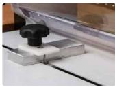
Micro switch is a sensor that will automatically trigger the punch when the paper is inserted into the die slot.For a more efficient workflow.
