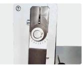
Punch 700 models come equipped with eccentric shafts. This feature allows the dies to be sharpened a few times.
