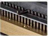
QSA (Quick Size Adjustment) technology allows the quick cancellation of punching pins without having to remove the die.(1)
