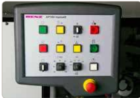
Manual control panel for setup.
