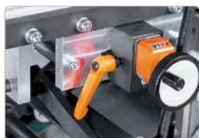
Manual lever adjustments for paper formats.
