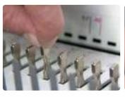
QSA (Quick Size Adjustment) technology allows the punching pins to be cancelled and the paper formats to be changed quickly and easily.<sup>(1)</sup>
