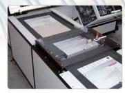
Optional extra: DBW 500 - conveyor flips the back cover into position.
