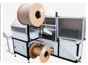
Spool de-winding with integrated paper separation re-winding
