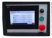
Menu-driven touch-screen control panel. Optional remote maintenance machine control module for remote diagnostics, software adaptations and connection to the internal company network.
