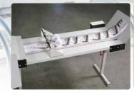
Optional extra: Shingle conveyor - height adjustable conveyor can be used in a continuous running function or with an adjustable overlap setting.
