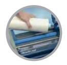
Film Loading Top Roll. Lift Heat Shield and simply insert film plug into colour coded cup and lock.
