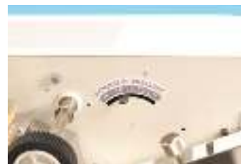
Separator pressure adjustment prevents double feeds.
